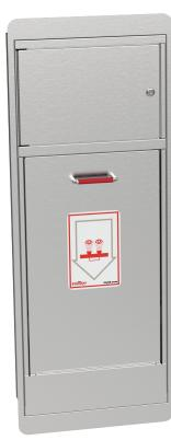
The T2236/T2536 emergency eye wash or eye/face wash station is a wall-mounted or recessed unit that includes an integrated mixing valve so that the plumbing can be run directly to the unit. The eye/face wash shall be manufactured of corrosion resistant materials. The integral valve assembly shall have ½" connections with check valves for hot and cold-water inlet connections. Unit shall include universal ANSI compliant sign.
