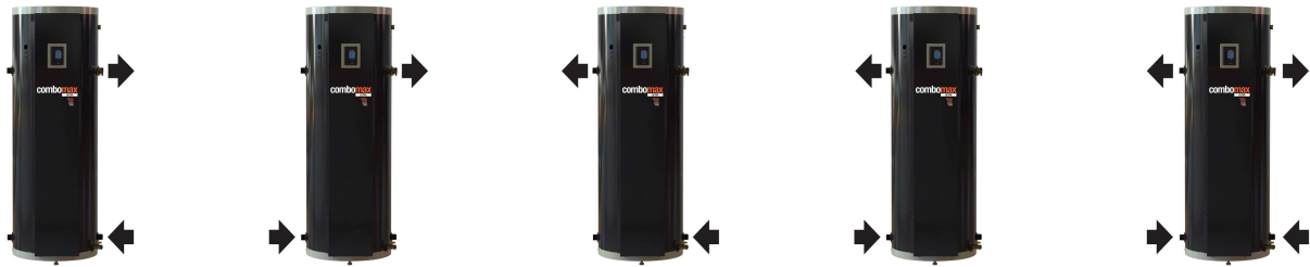
Figure 1: Possible installation configurations
